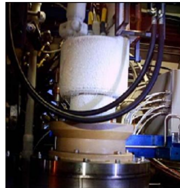
Determination of source of excessive frosting on the cryogenic subsystem & re-evaluation of safety valve size to withstand different accidental conditions etc.
