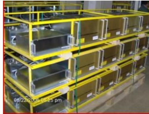
QHPS and LPU installed in LHC Quench Heater Power Supplies Local Protection Units
