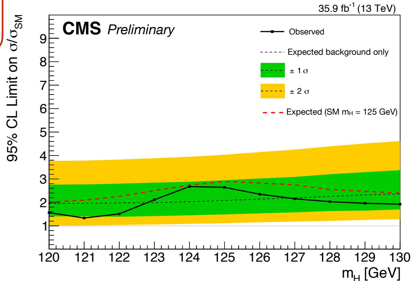
\* best fit is obtained for a signal strength of  $0.7 \pm 1.0$  at a Higgs mass of 125 GeV
