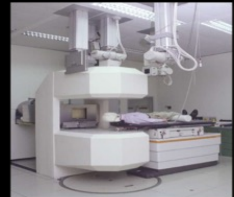
In-beam PET scanner at ^{12}\text{C} -therapy unit at GSI
