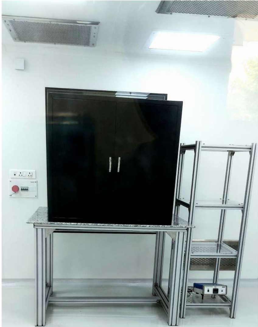
Probe station with dark box in clean room (class 1000)
