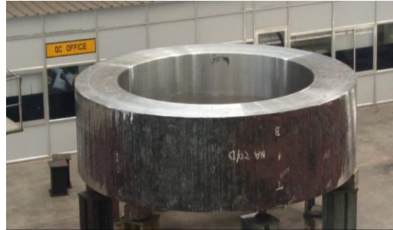
750 thick Ring Forging ( \Phi 3800 ID x 750 thk x 1200 L ; 100 t)
