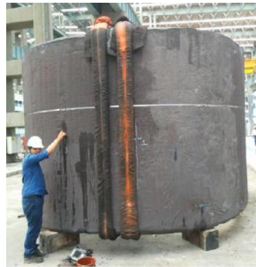
340 thick Shell Forging ( \Phi 4200 IDx340 thk x 3000 L ; 113 t)
